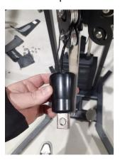
**STEP 55:** Attach the carabiner to the cable pull handle
