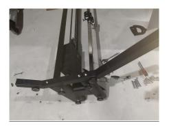
STEP 44: Thread the cable through the rollers
